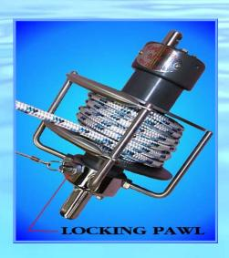
Another innovation of the Reef-Rite system is the use of a mechanical pawl. This is similar to the primary winches. The pawl, when engaged, allows the furler to rotate in only one direction. As a result, when a sail is furled the load is on the pawl and not on the furling line. The solid locking action of the pawl means improved sailing performance under furled conditions.
